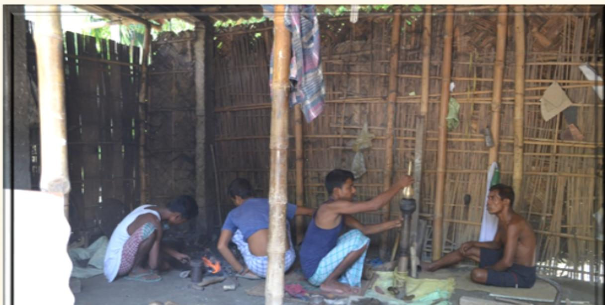
The melting furnace is a unique and important requirement in the process of manufacturing bell and brass metal products. The melting furnace or *Chula* is utilised for melting the raw material. The *Chula* is prepared by the unit owners in a traditional mode. It is about 40-70 cm wide and 15-60 cm deep. Hard coke is used for melting in the *Chula*.
